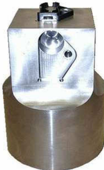
Sonotrode for continuous stress test with ultrasonic (automobile industry)
